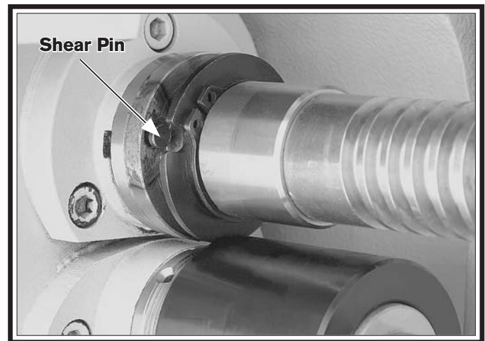
Figure 133. New shear pin installed in bore.
